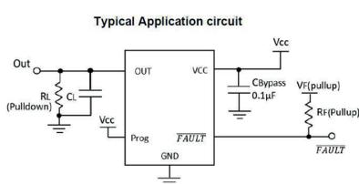
CL, CBypass and RL integrated on the sensor PCB
